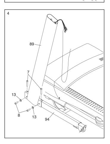
Identify the Left Base Cover (82) and the Right Base Cover (83). Slide the Left Base Cover onto the Left Upright (89). Slide the Right Base Cover onto the Right Upright (90). Do not press the Base Covers into place yet.
